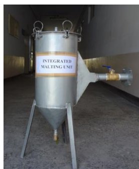
Fig 1(a) Integrated Malting Unit Fig 1 (b) Line diagram of Integrated Malting Unit
